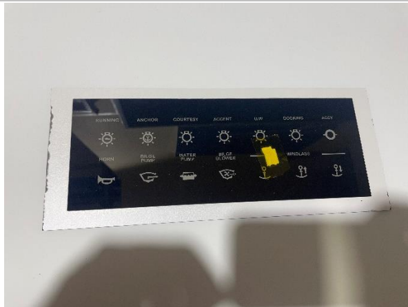
Figure 2.4 - UUT After Solar Radiation Test
