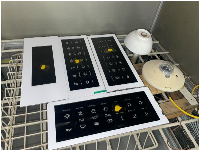
Figure 2.2 - UUT Inside Solar Radiation Chamber
