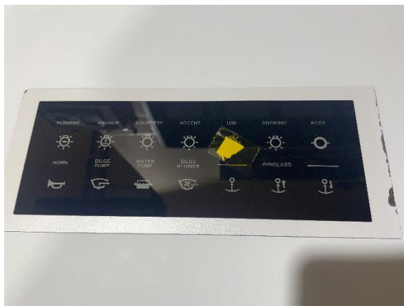
Figure 2.3 - UUT After Solar Radiation Test
