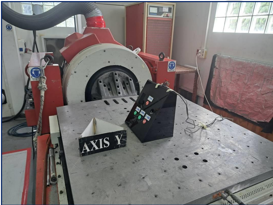
Photograph 6.1.5 Random vibration test setup (longitudinal axis)
