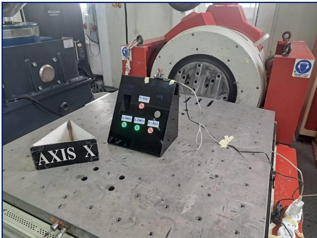
Photograph 6.1.3 Random vibration test setup (transverse axis)
