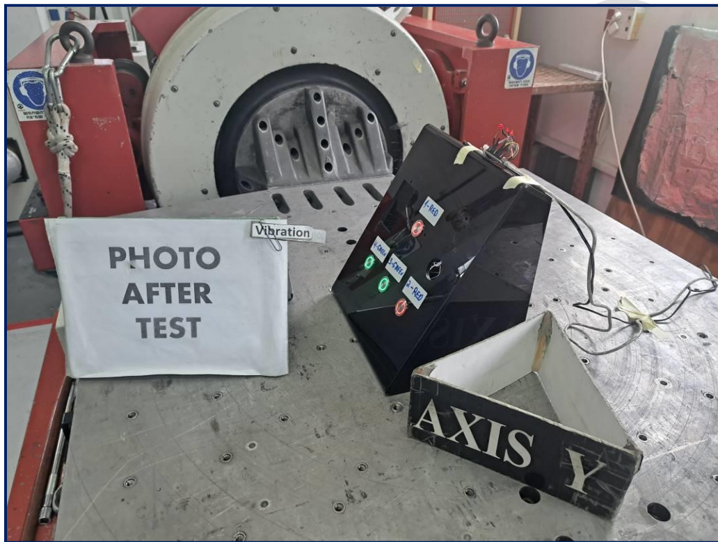
Photograph 6.1.6 The EUT functional check after random vibration (longitudinal axis)
