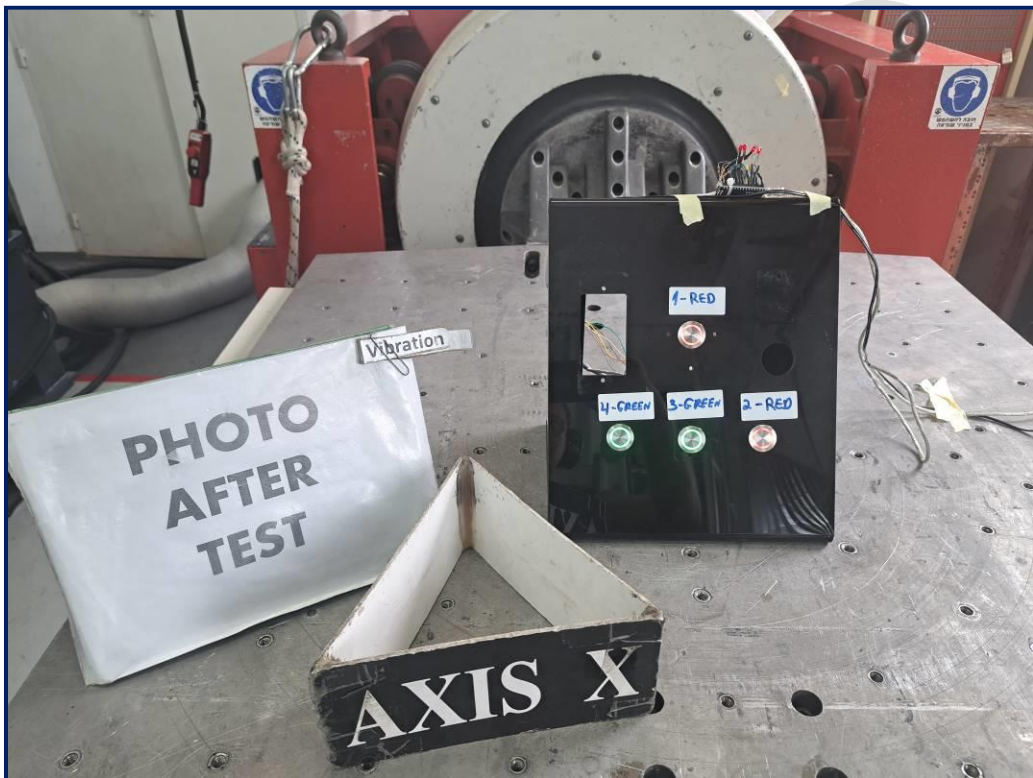
Photograph 6.1.4 The EUT functional check after random vibration (transverse axis)
