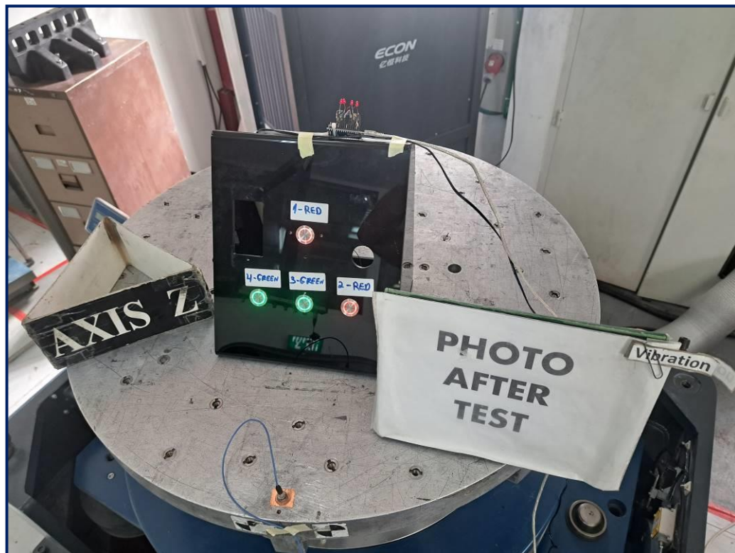
Photograph 6.1.2 The EUT functional check after random vibration (vertical axis)
