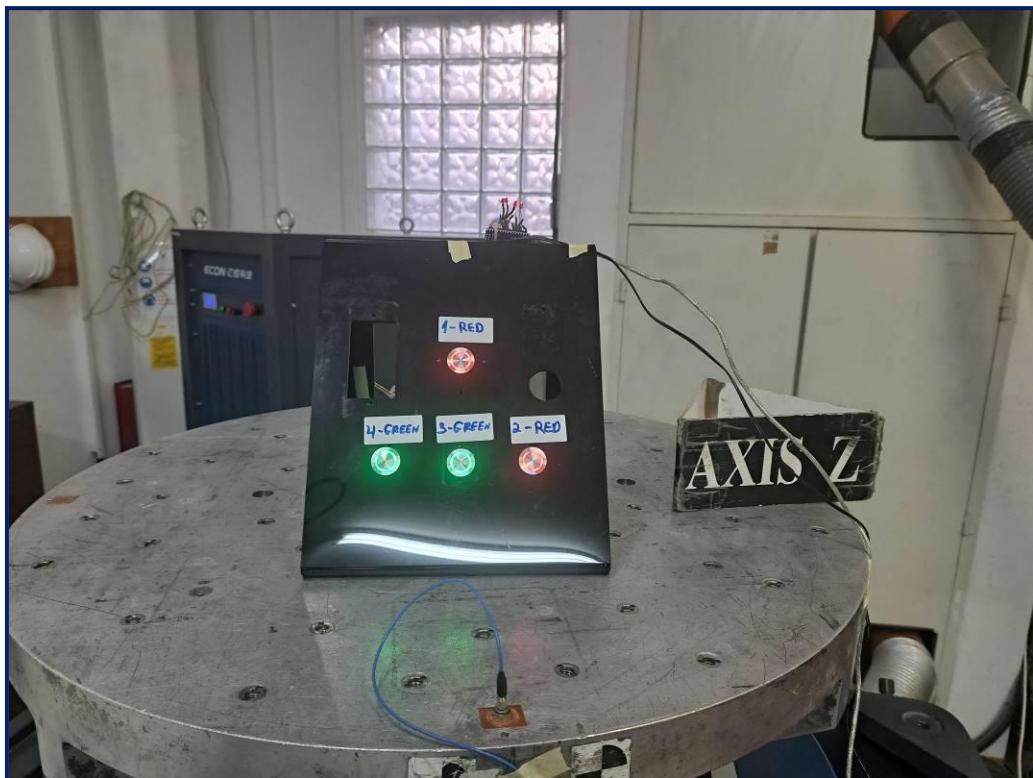
Photograph 6.1.1 Random vibration test setup (vertical axis)
